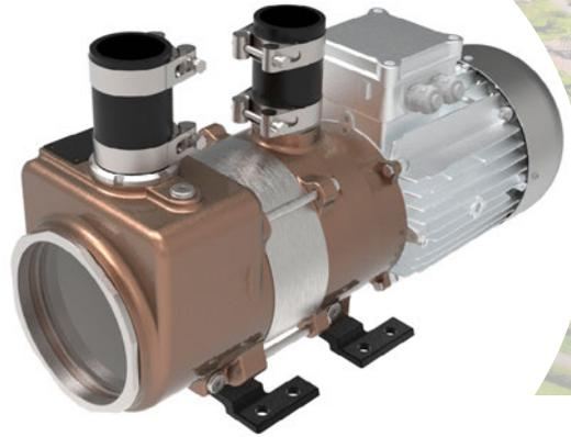
The Winter vacuum sewage water pump (WVSP) is designed for the conveyance of sewage water, including grey and black water. The integrated cutting mechanism effortlessly shreds solid components such as wet wipes, baby wipes, and fecal matter. Due to its construction, the liquid ring vacuum pump is particularly robust and easy to maintain, ensuring reliable and safe operation at all times. Typical applications include toilet and sanitation systems on ships and in buildings.
