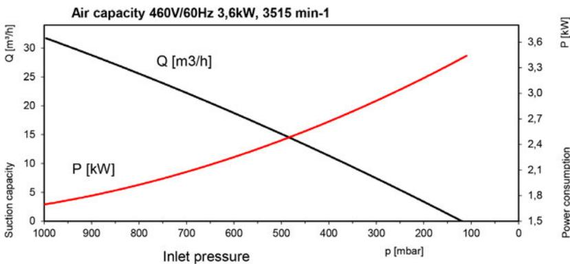
Under different operating conditions (e.g., different data of the gas to be conveyed or the operating fluid, co-conveyance of additional fluid, conveying of gas-vapor mixtures), the characteristics may change.
