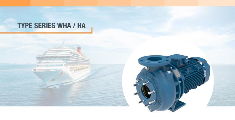
Sewage pumps type series WHA and HA are single-stage, end-suction centrifugal pumps specifically designed for the conveyance of sewage water and other solid-laden fluids. They are characterized by their robust construction and high efficiency. These pumps feature impellers with a large free passage, allowing solids to be transported through the pump without causing clogging.
